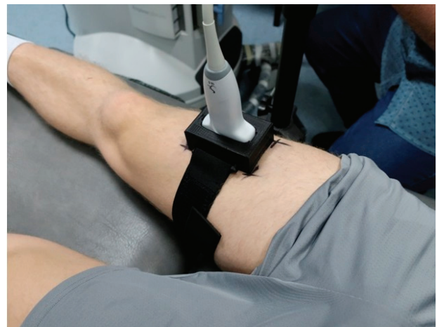
Fig. 2. Measurement of muscle stress with the use of an attachment to hold the USG scanner head – right lower limb
